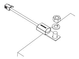
3. Route the sensor cable to the charger and plug it into the Bank 1 (default if using only one BTS), Bank 2 or Bank 3 connector on the rear panel. It may be advantageous to temporarily apply a layer of tape around the connector to protect its locking tab from catching on something during pulling and routing.
